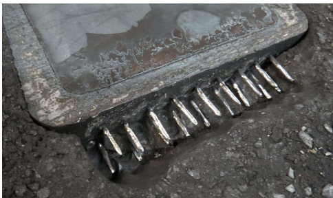
Cathode Nails: the only cathode assembly technology to reduce contact resistance
